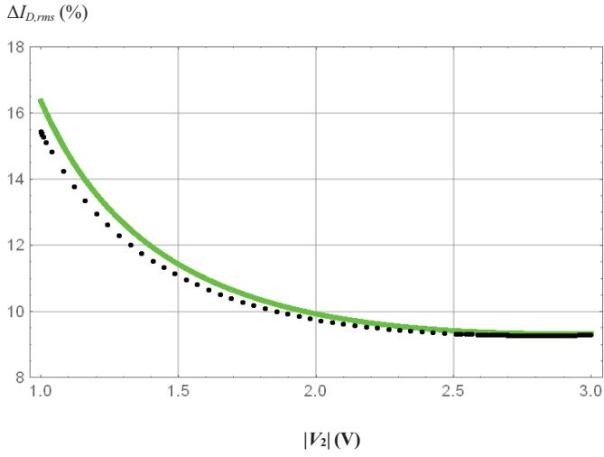
Fig. 4. The comparative plots of  $\Delta I_{D,rms,M}$  and  $\Delta I_{D,rms,SPICE}$  against  $|V_2|$
