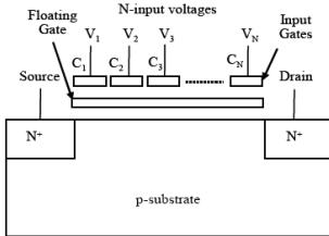
Fig. 1. A cross sectional view of N-type  $N$  input FGMOSFET [8], [15]
