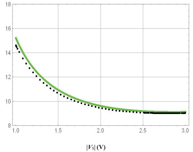
Fig. 3. The comparative plots of  $\Delta I_{D,rms,M}$  and  $\Delta I_{D,rms,SPICE}$  against  $|V_1|$
