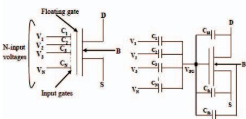
Fig. 2. The symbol (left) and equivalent circuit model (right) of an N-type  $N$  input FGMOSFET [8], [15]
